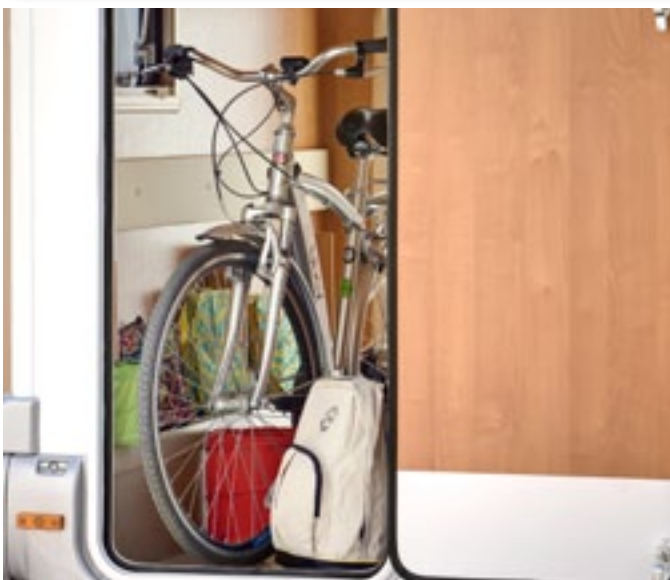
Variable volume rear storage with fold-up lower bunk and exterior access from either side.
